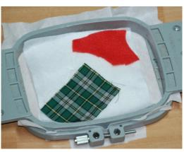
5. Return the hoop to the machine and stitch the next two colours. Here you can see the stitching plainly on the plaid fabric, but it may be harder to see on the red. Pause the machine and again remove the hoop without unhooping the design.
