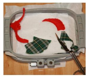
Return the hoop to the machine and continue stitching, pausing the machine before the second last colour (the outline). Remove the hoop, but do not unhoop the design.
