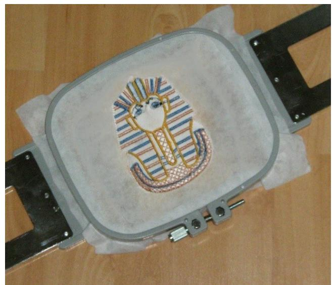
8. Place the second piece of felt on the back of the hoop so that it completely covers the stitching. Tape the corners to keep it in position, as I have done here.
