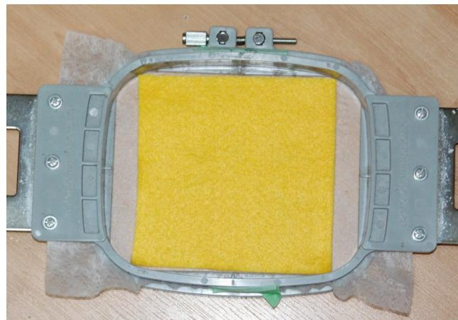
5. Place the hoop in the machine and stitch the design up to the second-last colour. Pause the machine before the final thread colour stitches.
