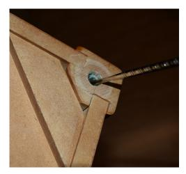
I scraped out as much as I could of the old glue from the previous repair. I'm using a nut pick as a tool for this purpose.
