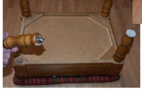
The problem was that the wood had deteriorated around the insert nut – the bit that holds the leg
