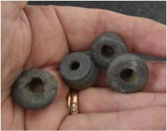
Unfortunately, the original rubber feet can crumble over time, or actually soften and "melt" from exposure to sewing machine oil.
