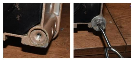
Lining up the end of the screwbolt with the screwhole in the bottom of the machine, I place the foot in position. It has an adhesive back, so it will stick in place. I then push on the bolt with my screwdriver until it makes contact and can be tightened into place. This process takes a bit of fiddling, but once you get the hang of it, you can install a set of these silicone bumpers in only a few minutes.
