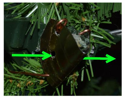
It would have been easier to drill or punch these holes before the bracket was attached to the tree, except that I need them to align so I can push through the pin that I'll use as a pivot. There was no choice but to drill through after the bracket was in place on the tree. It's awkward, but it's the only way to be sure the holes will align.
