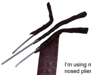
I've wrapped all three wires, leaving a tail of the tape on one of them, which I'll use to finish wrapping the group once I've twisted them together.
